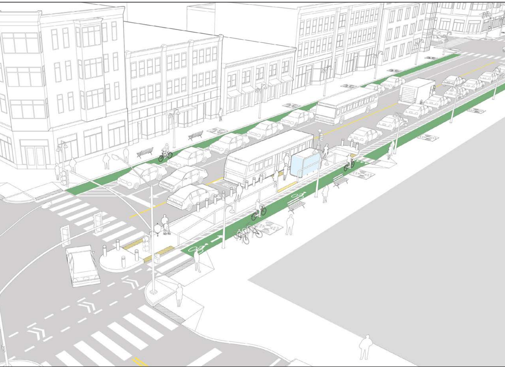
Figure 16: The National Association of City Transportation Officials (NACTO) has developed design guidance for “Transit Streets” that prioritize bus operations. (Image source: NACTO.org)
